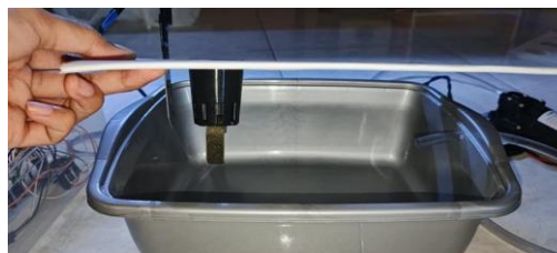
Figure 6. Placement of the Soil Moisture Sensor in the Planting Container
