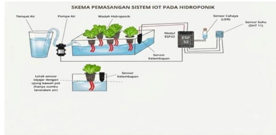
Figure 4. Layout of the IoT System in the Planting Container
